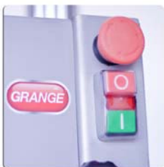
Emergency Cut Off Switch
